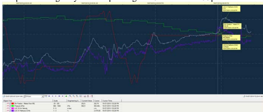
Graphs showing Inbye sensor peaking at 2.5% CH4 at 1:53pm
